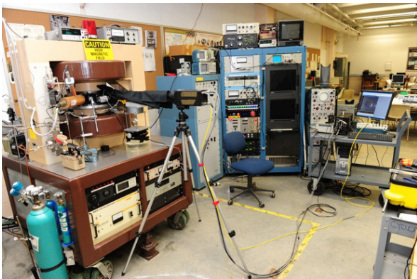
Figure 2: PI-MAX camera imaging fast phosphor screen.
